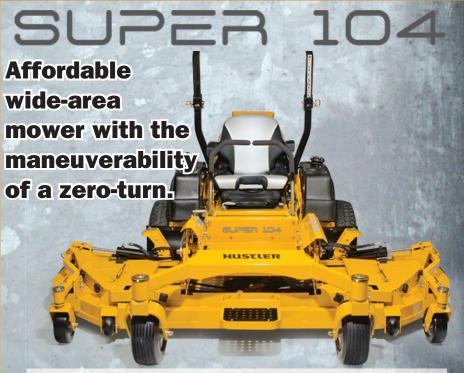
With premium engine options & 104" cutting width, the Super 104 can mow up to 84 acres in 8 hours at 10mph and will mow where most wide-area mowers cannot.
