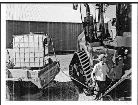
Filling the DEF tank is easy. The DEF tank in 2011-2012 Case IH high-horsepower tractors is sized so that it needs refilling every other fuel fill.
